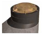
WrapidSeal<sup>™</sup> manhole encapsulation system consists of an engineered primer and a unique, wrap-around, heatshrinkable sleeve designed specifically to seal joints and prevent groundwater from entering a collection system. WrapidSeal<sup>™</sup> can be utilized on both new construction and rehabilitation of existing manholes.
