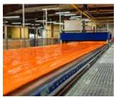
The Omega UV Liner is constructed with ECR (corrosion-resistant) fiberglass and advanced UV resins – proven to be one of the strongest on the market. Omega Liners are manufactured using unsaturated polyester or vinyl ester resins for environmentally conscious projects and are offered from 6" (150mm) to 66" (1675mm).
