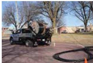
HydraBed Reel Management system is an integrated bed design with an unmatched 5000-pound lift capacity that eliminates the need for a reel trailer. The new Reel Lift system combines the functions of reel pickup and transport with semi-autonomous hydraulic cable payout, retrieval, and figure-eight deployment in one compact, truck-bed-based package.
