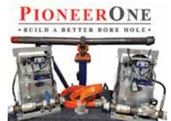
While averaging 4000 feet per bit, our newly designed 2", along with our 3" and 4" HDD Air Hammers, run on a 200/400 compressor with ease. Save on your fuel bill and run a smaller compressor.
