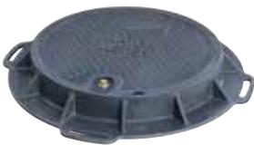
Trumbull Manufacturing composite manhole frames and covers offer superior corrosion resistance to H2S gas and are lighter weight compared to cast iron. Other benefits include AASHTO H20 & H25 traffic rating and O-ring sealed for water infiltration. Trumbull also offers wall sleeves and Link-Seal® for creating and sealing wall penetrations in concrete vaults and other underground boxes.
