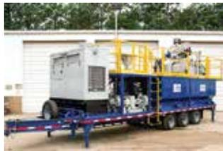
Triflo's MFS 3000ti Mud Mixing and Cleaning Machine with 3800 gallon two compartment tank integrated into a triple axle trailer. The system includes Triflo's 4" hopper with in-line jetting, swivel mud guns, Triflo's 148L-6 Double Deck Shaker with a Triflo 8/4 single manifold Mud Cleaner, two Triflo 3x4x30 HP centrifugal pumps, one Triflo 3x4x20 HP centrifugal pump and one watertight central control panel.
